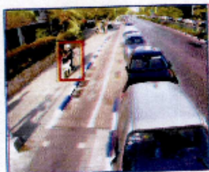
Real-time detection (anomaly detection) of a motorcycle in pedestrian-only zone
